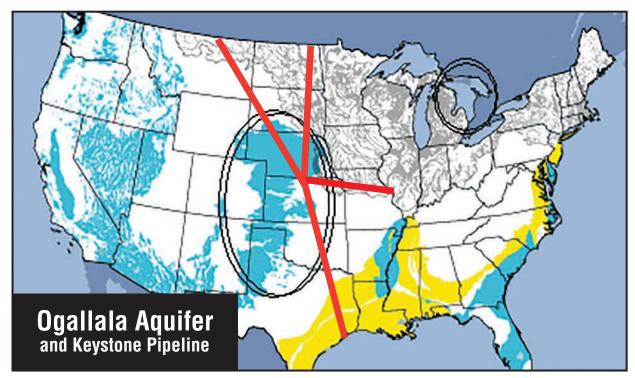
This U.S. Geological Survey map shows the Ogallala Aquifer (center, circled). It holds as much water as Lake Huron (circled, top). BLUE: Unconsolidated sand and gravel aquifers near the land surface. YELLOW: Semiconsolidated sand and gravel aquifers. GRAY: Sand and gravel aquifers of alluvial and glacial origin. RED: Projected Keystone XL routes.
